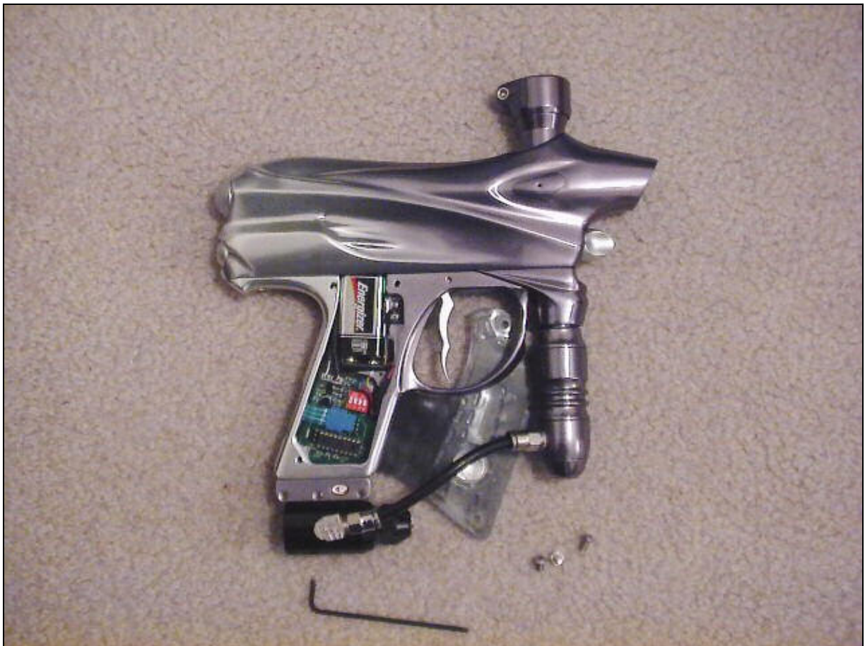
Figure 1 – Grip cover screws removed and grip panel folded back
